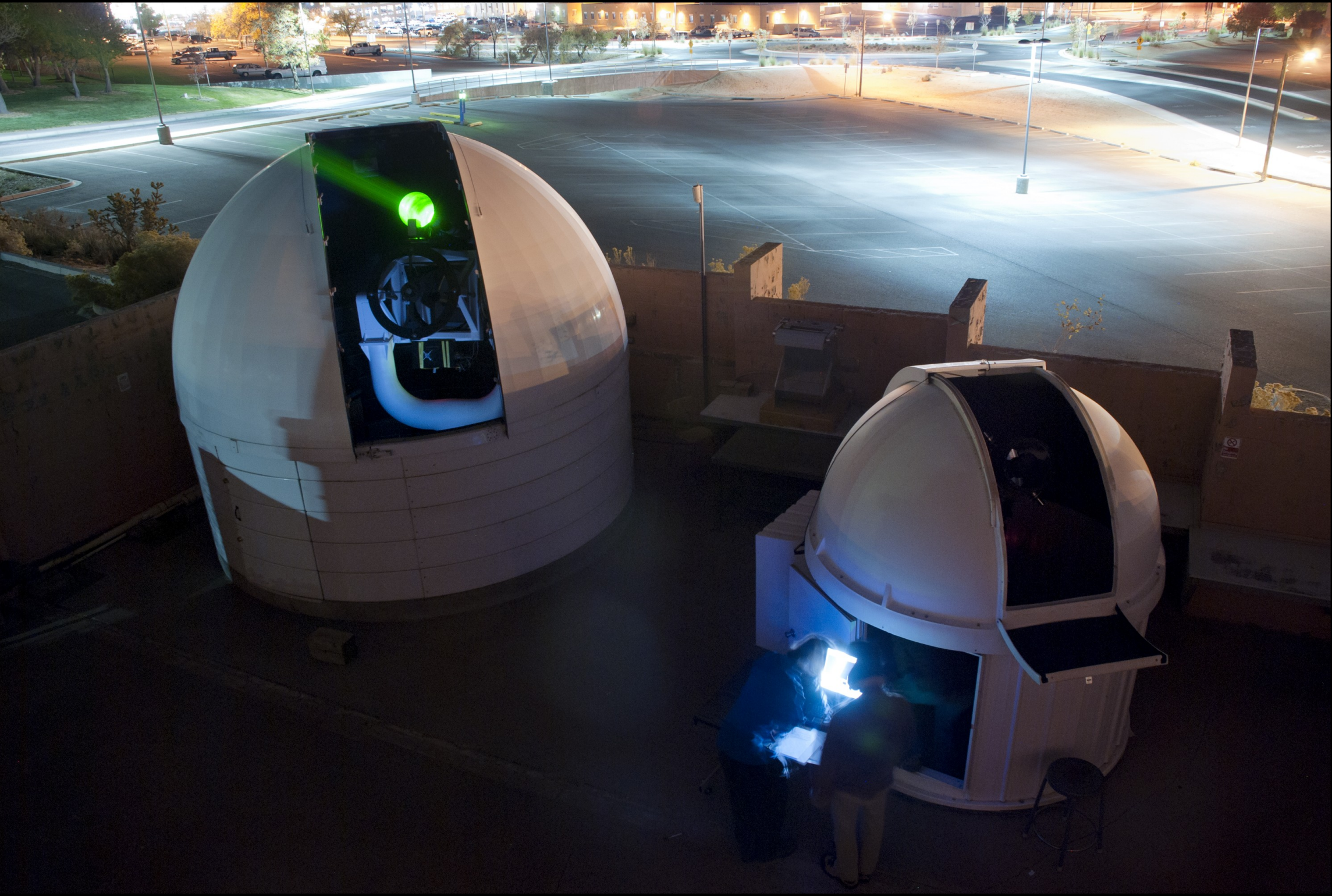
Figure 2 - A picture of the UNM Campus observatory shown during the combined observing campaign. The large dome on the left houses ALE, the smaller dome to the right houses a small wide-field photometric telescope and the ASIVA camera system is the small gray box behind and between the two domes.
