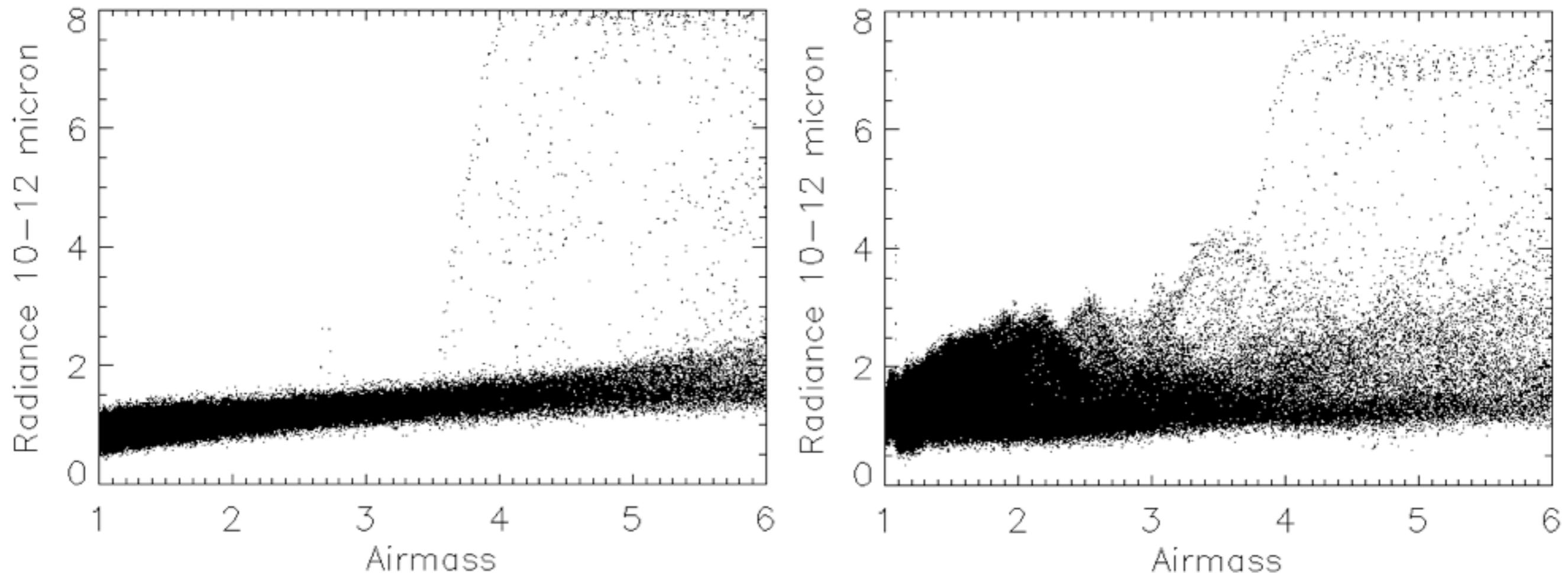
Radiance vs. airmass for the two images shown before. The high scatter of the lower envelope in the left (clear sky) image is a sign that the instrument needed re-calibration.
